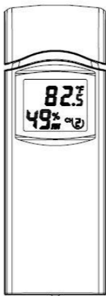
Figure 1: Multi-channel Thermo-Hygro Sensor
