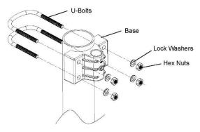
Figure 8: Sensor package mounting diagram 5-1
