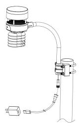
Figure 12: Sensor package mounting diagram 5-5
