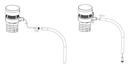
Figure 9: Sensor package mounting diagram 5-2
