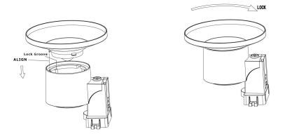
Figure 15: Rain collector top installation diagram
