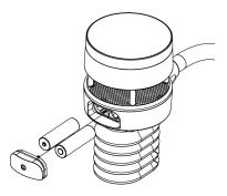
Figure 7: Battery installation diagram
