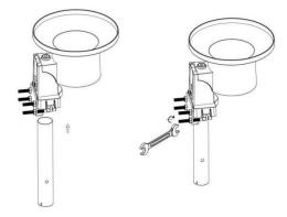
Figure 17: Rain gauge installation with U-bolts
