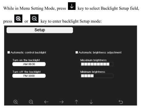
Figure 31: Backlight Setting Screen
