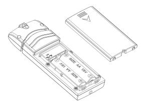
Figure 19: Indoor sensor battery installation
