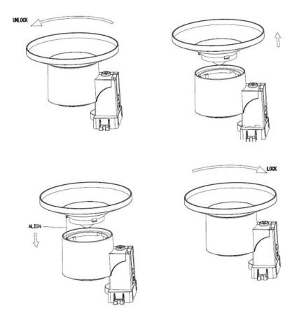
Figure 36: Rain gauge maintenance
