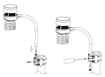
Figure 11: Sensor package mounting diagram 5-4
