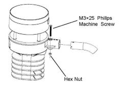
Figure 10: Sensor package mounting diagram 5-3
