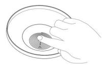
Hook the filter hook on the edge to install.
